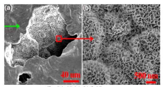
图 2 堇青石微孔表面水滑石层 (LDHs) Figure 2 Hydrotalcite layers on cordierite microporous surface
