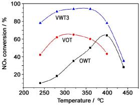
图  $6\,WO_3$  对  $V_2O_5$ -TiO<sub>2</sub>/PRD 催化活性影响 Figure 6 Effect of WO3 on the catalytic activity of  $V_2O_5$ -TiO<sub>2</sub>/PRD
