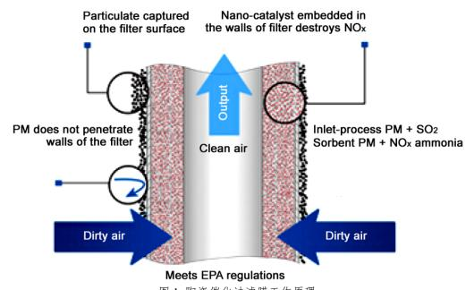
图 1 陶瓷催化过滤膜工作原理 Figure 1 Working principle ceramic catalytic filtration membrane
