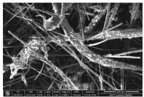
图 5 纤维表面催化剂负载显微结构 Figure 5 Microstructure of catalyst supported on the fiber surface
