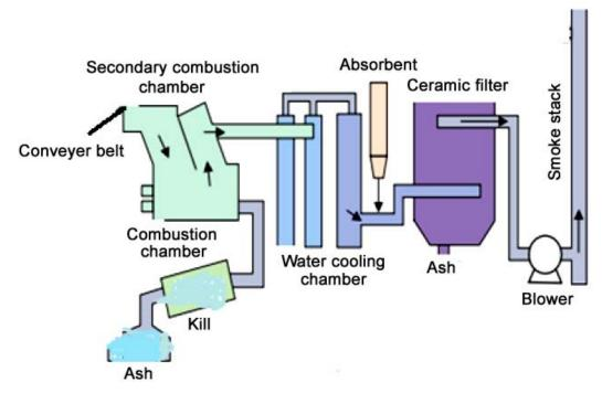
图 8 垃圾焚烧气体净化流程 Figure 8 Gas purification process for waste incineration
