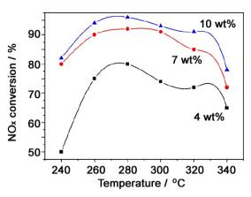
图 7 不同催化剂负载量的纤维膜脱硝效率 Figure 7 Catalytic efficiencies of fiber membranes with different catalyst amounts
