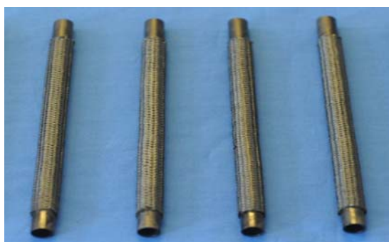
图 20 PIP- \text{SiC}_f/\text{SiC} 复合材料包壳 Figure 20 \text{SiC}_f/\text{SiC} composite fuel rod cladding fabricated by PIP process
