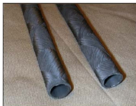
图 21 多层结构 \text{SiC}_f/\text{SiC} 复合材料包壳管 Figure 21 \text{SiC}_f/\text{SiC} composite fuel rod cladding with multilayer structure
